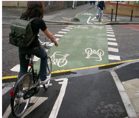
An example of a cycle crossing using elephant footprints and coloured surfacing (although in York, for a non-priority crossing, the surface would be red)
