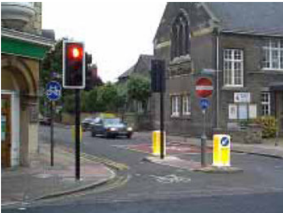
An example of a simple one-way 'plug' (in Cambridge).
